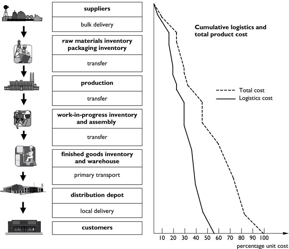
**Figure 1.4** A typical physical flow of material from suppliers through to customers, showing stationary functions and movement functions, linked to a diagram that reflects the 'value added' nature of logistics
